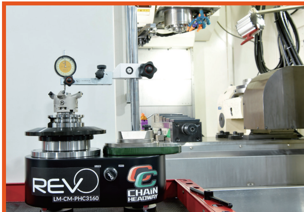
機台外測量，不占用主軸時間 Do measurement in advance. Reduce cnc machine down time.
