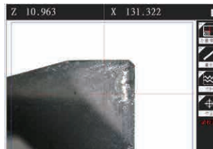
開啟正光，可檢視刀具刀口表面實際狀態 Turn on the positive light, you can view the actual state of the cutter edge surface
