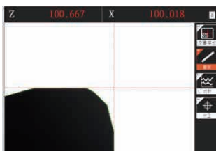
具動態十字線，可精準定位刀尖位置 With dynamic crosshairs, the position of the tool tip can be accurately positioned
